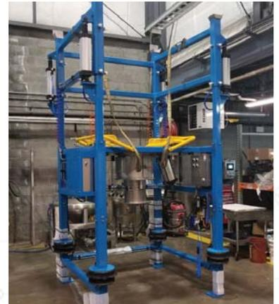
and protective features like bellows for the load cells and a cap for the bag sealing nozzle to cover when not in use.
