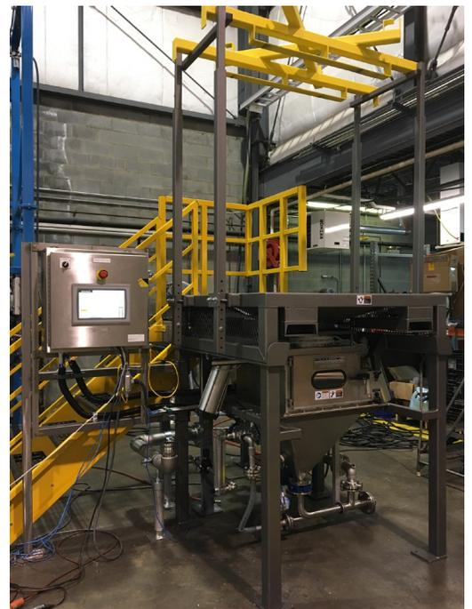
*Dual modules: small bag discharge (top) and bulk bag (FIBC) discharge (bottom)*
