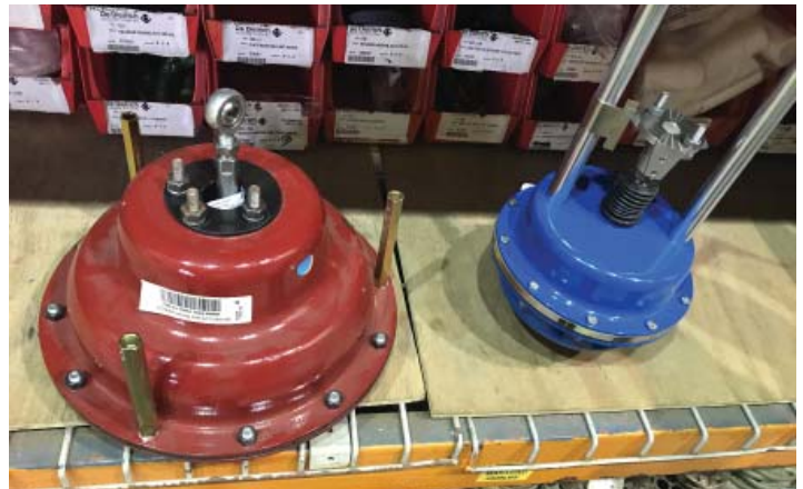
Standard “red” actuator and high pressure “blue” actuator
