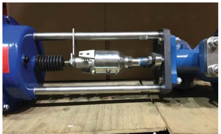
High pressure actuator with pneumatic coupling
