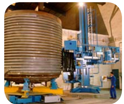
AN APPROPRIATE TOOL: AUTOMATED WELDING = ENHANCED LIFESPAN, ERADICATION OF BUTT WELDS
