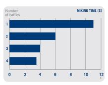
CHANGES IN PUMP FLOW AND MIXING TIME DEPENDING ON THE NUMBER OF BAFFLES (CALCULATED FOR A 1600-LITRE OPTIMIX®)
