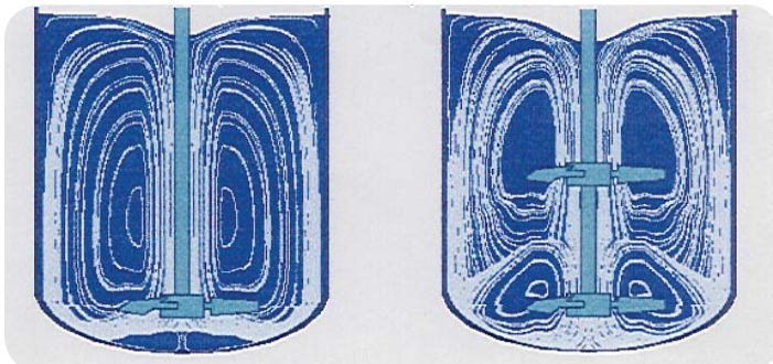
Comparison of pumping capacity: single versus dual tier hydrofoil blades. Greater pumping capacity equals reduced batch mixing time.
