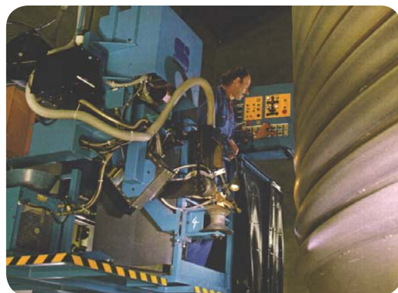
Half-pipe coils being attached using automated welding machine.
