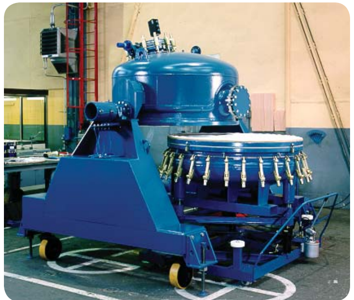
Special Portable Nutsche Filter with pneumatic lowering bottom and perforated plate with casters. This design also features a pivoting top head to ensure complete cleaning for pharmaceutical environments.
