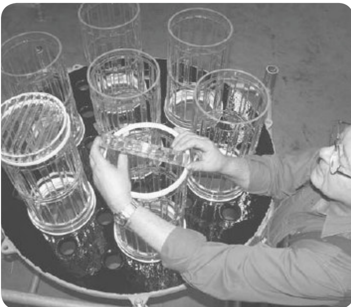
Fig 1: CORE-TRAY DIN 1000 assembly, here for packing with glass support.
