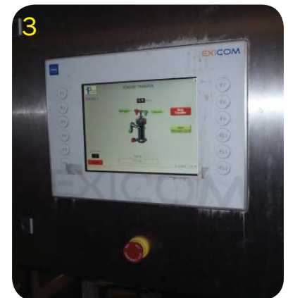
1/2. Powder Pump installation on reactors. 3. PLC control system with HMI graphic displays.
