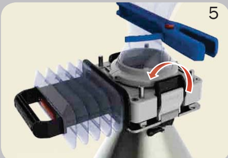
5 Active half lowered over integrated Spigot sealing against Passive Valve creating full containment.
