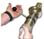
from the sample valve when the syringe is offered up to its mount using a pin and cam arrangement. When the syringe is released the sample valve and syringe automatically close preventing any release of fumes or product. The sample is contained within a borosilicate glass tube contained within a sturdy stainless steel carrier. The syringe can then be taken to the lab and safely dispensed using the syringe dispensing attachment.
