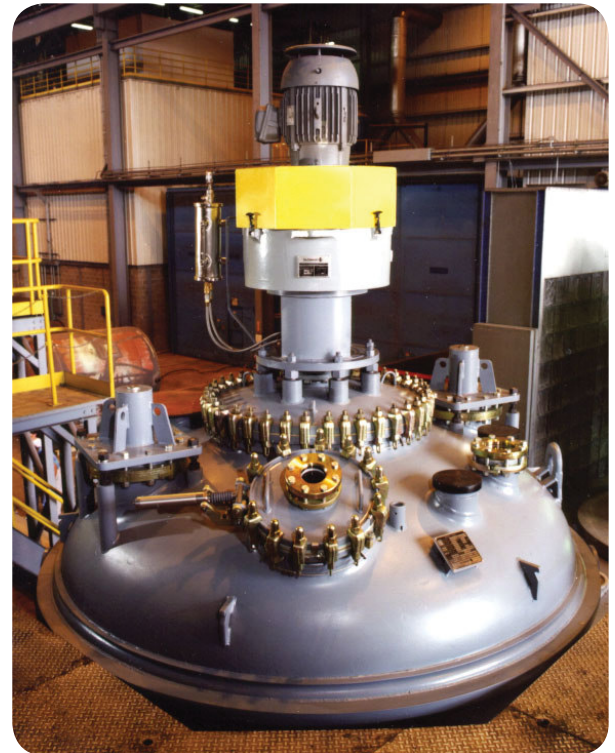
Series 60 drive, shown here on a closed welded SA series reactor.
