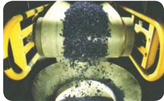
Enamel being prepared for reglassing process
