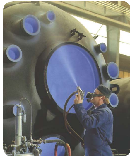
Enamel is sprayed like paint on the surfaces to be glass-lined
