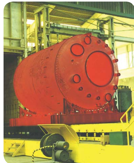
Vessel is fired at high temperatures in an electric furnace
