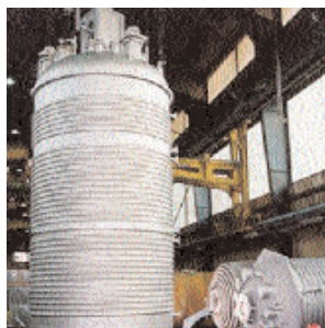
Left: 4,000 gallon OptiMix® reactor
