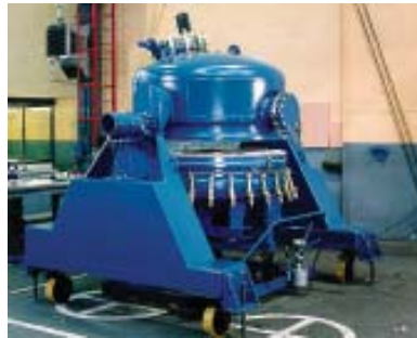
Left: A special portable Nutsche filter with pneumatic lowering bottom and perforated plate with casters
