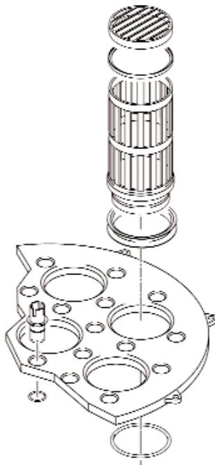
Fig.: CORE-TRAY column packing support with support grid on top for random packing and with distributor nozzles
