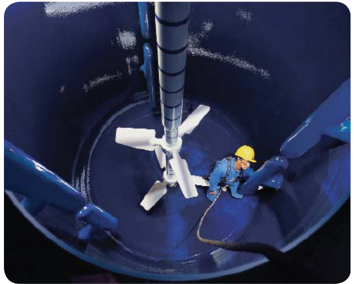
Three sidewall-mounted baffles of this 4,000-gallon (15,100 liter) Optimix reactor reduce mixing time by one-third. Reductions in vortexing minimize the amount of product that dries and sticks to reactor wall, and can eliminate splashing of the reactor head. Shown with GlasLock agitator with two tiers of HydroFoil blades.
