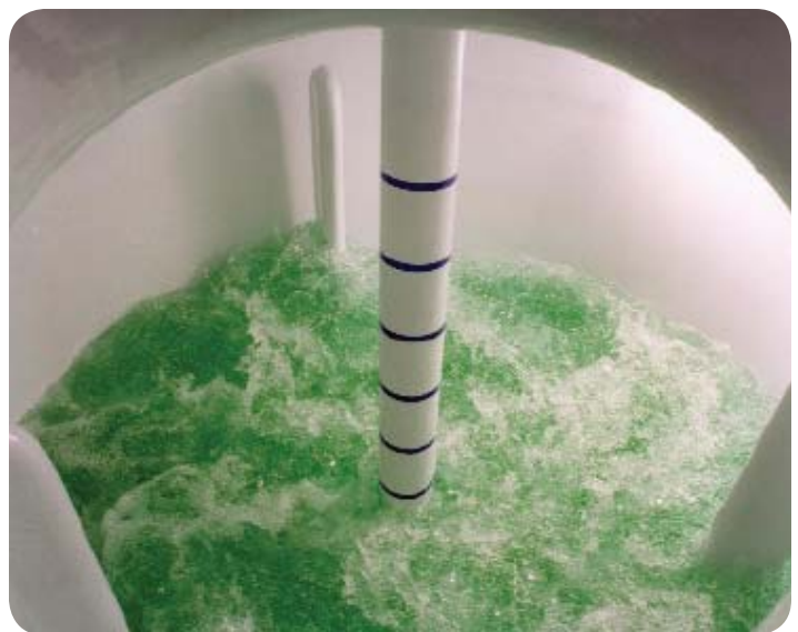
Compared with a single baffle extending downward from a flange located at the top of the vessel, the tri-baffle design creates significantly greater turbulence, thereby improving mixing efficiency, solids suspension, and heat and mass transfer.
