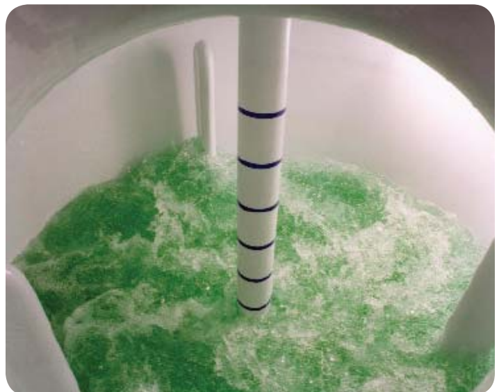
Three sidewall-mounted sets of baffles reduce vortexing and splashing of the reactor head, and minimize the amount of product that dries and sticks to reactor wall, while reducing mixing time by one-third.
