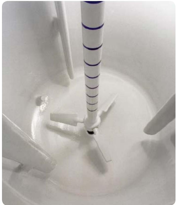
Three baffles are used in OptiMix reactors to match the number of agitation blades, canceling radial stresses that would otherwise be incurred by the hub.
