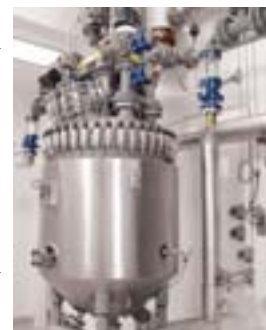
The OptiMix® wall-mounted baffle design frees up room on and around the 200 gallon reactor head permitting more ports for process analytical technology.
