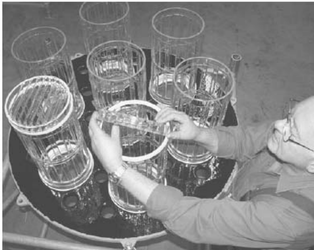
Fig 1: CORE-TRAY DIN 1000 assembly, here for packing with glass support
